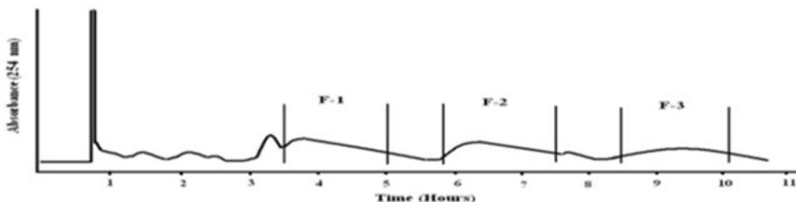
**Figure 2:** HSCCC separation 2 of theaflavin crude extract from black tea (254 nm), Solvent system Hex:EtOAc:MeOH:water (1:5:1:5) elution 2.0 mL/min, 800 rpm, sample size 200mg
