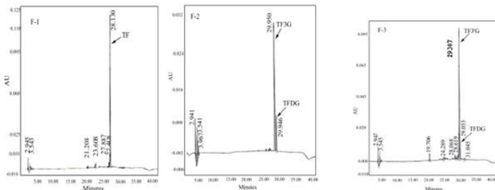
**Figure 3:** HPLC traces of fractions F-1, F-2, F-3 after HSCCC separation-1 using solvent system B Hex:EtOAc:MeOH:water (1:4:1:4)
