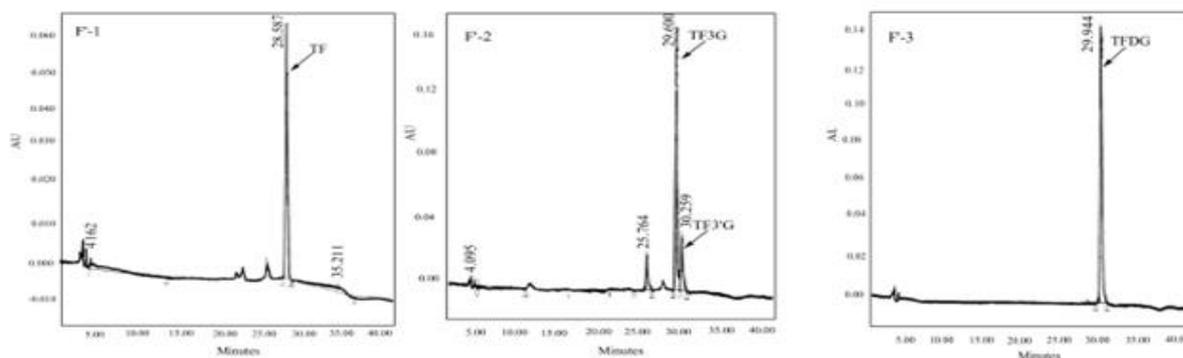
**Figure 4.** HPLC traces of fractions F<sup>-</sup> 1, F<sup>-</sup>2, F<sup>-</sup> 3 after HSCCC separation- using the solvent system C Hex:EtOAc:MeOH:water (1:5:1:5)
