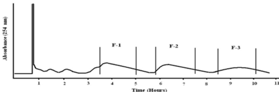
**Figure 1:** HSCCC separation 1 of theaflavin crude extract from black tea (254 nm), Solvent system Hex:EtOAc:MeOH:water (1:4:1:4), elution 2.8 ml/min, 1000rpm, sample size 200mg
