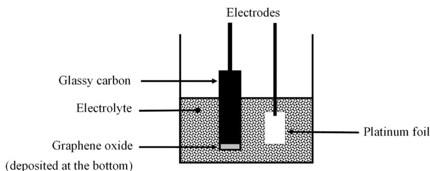
**Figure 8:** Electrochemical cell for extracting graphene oxide from bulk glassy carbon (Nasibulina *et al.*, 2010).
