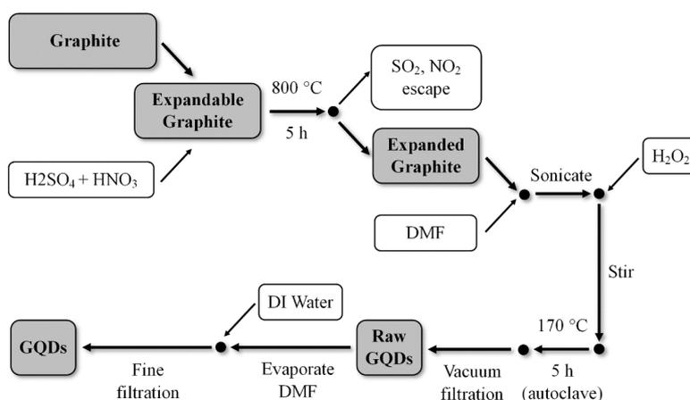
**Figure 7:** Flowchart of the solvothermal synthesis of graphene quantum dots from graphite using hydrogen peroxide as the oxidant (Tian *et al.*, 2016; Bandara *et al.*, 2022a).
