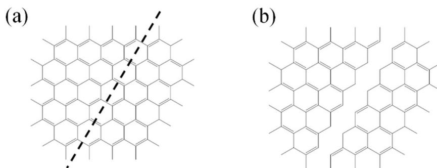
**Figure 5:** Hydrothermal cutting (deoxidization) of graphene. (a) before, and (b) after (Bandara *et al.*, 2022a).
