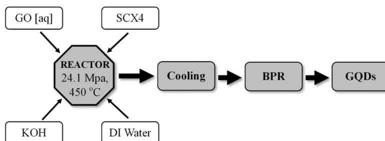
**Figure 6:** Flowchart of the continuous hydrothermal flow synthesis of graphene quantum dots from graphene oxide (GO) and calix[4]arene tetrasulfonic acid (SCX4) (Kellici *et al.*, 2017; Bandara *et al.*, 2022a).
