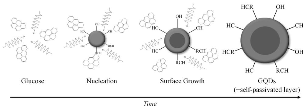
**Figure 3:** Microwave-assisted hydrothermal synthesis of graphene quantum dots from glucose precursor (Tang *et al.*, 2012).
