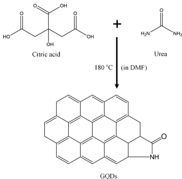
**Figure 4:** Solvothermal synthesis of pyrrolic nitrogen-doped GQDs (pN-GQDs), starting from citric acid (carbon source) and urea (nitrogen source) (Noor *et al.*, 2018).
