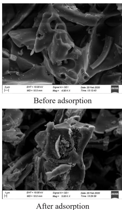
Figure 03: SEM images of adsorbent before and after adsorption of \text{Cu}^{2+} .
