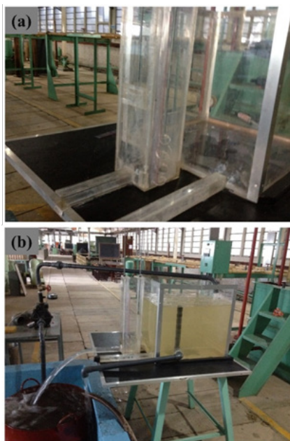
Figure 4: (a) The prototype model of lake, Bissokotuwa , and sluices (b) releasing water by maintaining reservoir head at constant.
